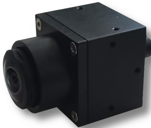
Figure 1: logiCAM-FPD3-AR0231 2.3 MP HDR Automotive Video Camera
